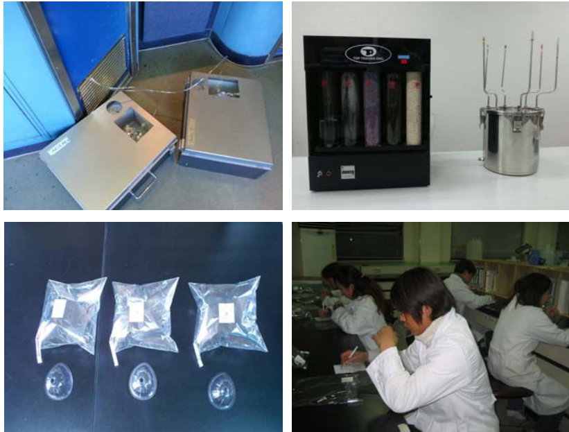
Fig. 1 Photograph of experimental device and estimation of odor samples by air dilution olfactory method.
