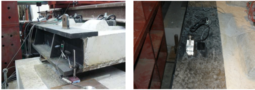
Fig. 4 Photograph of sensor instrumentation(acceleration and strain gauge)
