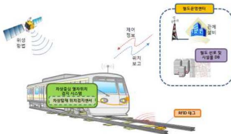
Fig. 1 Train position detection system
