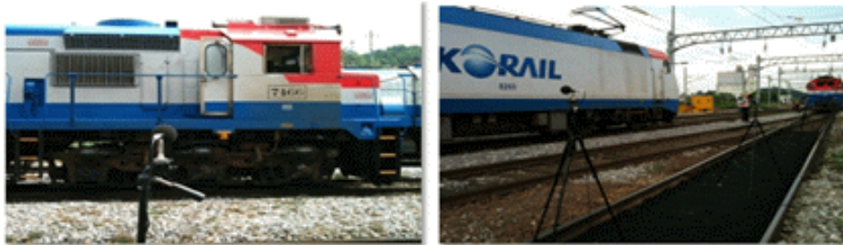
Fig. 1 Measurement of DL / EL Braking Noise
