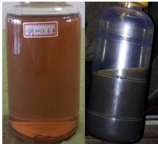
**Fig. 5** New and used reduction gear oil
