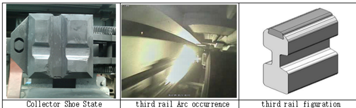
Fig 2 Power Collector Shoe and third rail
