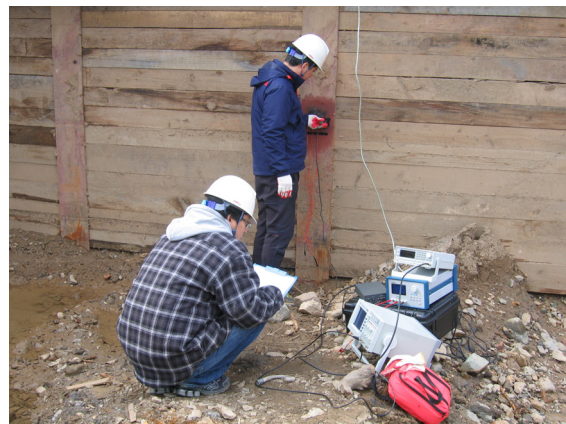
Fig. 8 Measurement probe of magnetic anisotropy sensor
