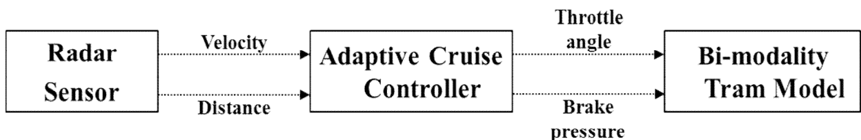
Fig. 3 Configuration of adaptive cruise controller
