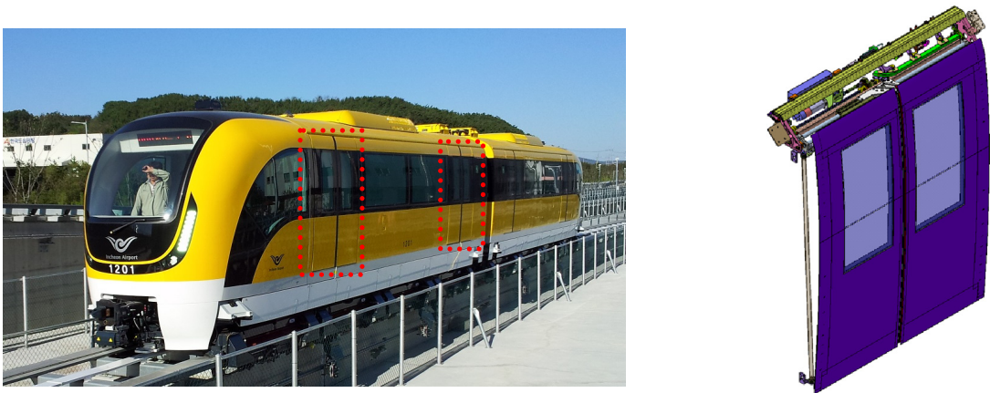
Fig. 1 The basic shape of the passenger entrance doors of MAGLEV
