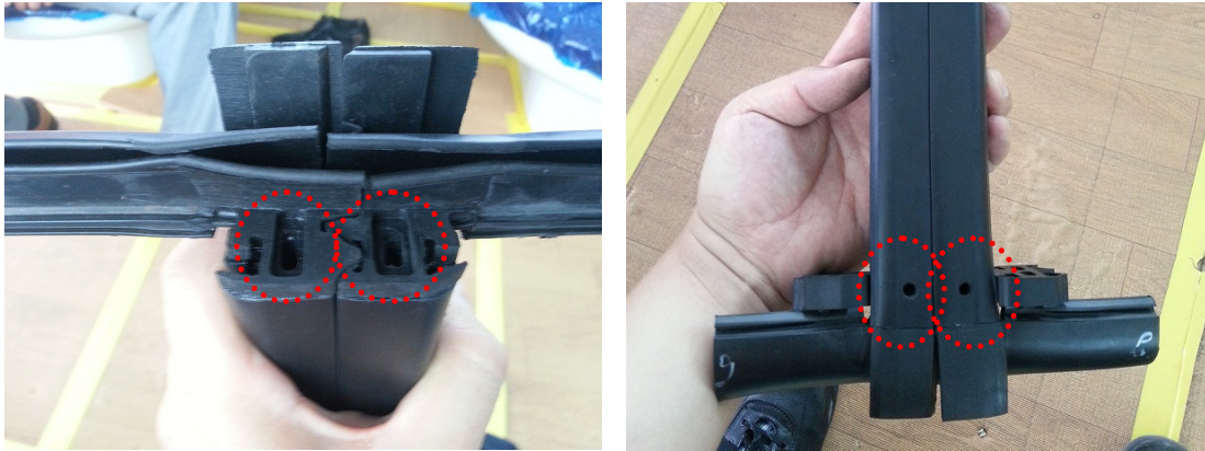
Fig. 5 The shapes of drain holes on the center rubbers (Upper / Lower : Sample parts)
