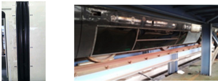
Fig. 4 Side faring and bogie cover for reduction of aerodynamic drag
