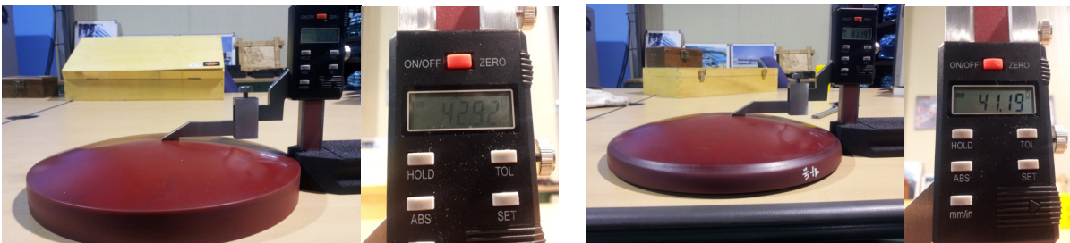
Fig. 10 Extreme vertical load test before (left) and after (right) the shape
