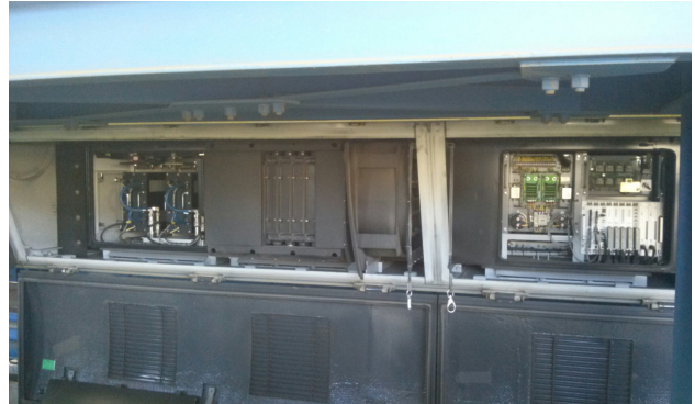
Fig. 5 Propulsion System Mounted on Prototype Train
