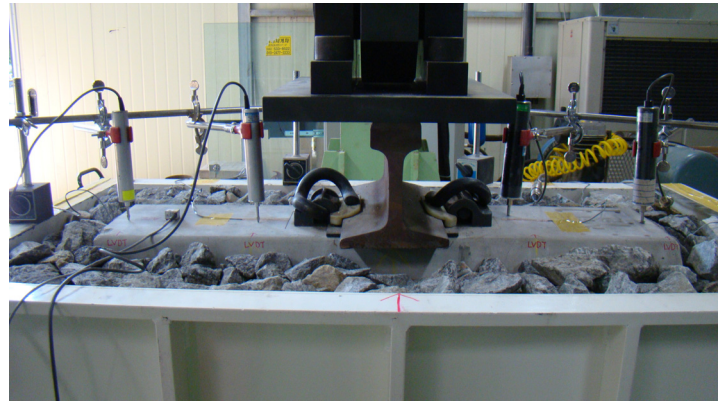
Fig 4 Installation of LVDTs
