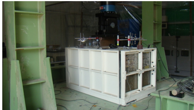
Fig 1 Repetitive load test with prismatic chamber
