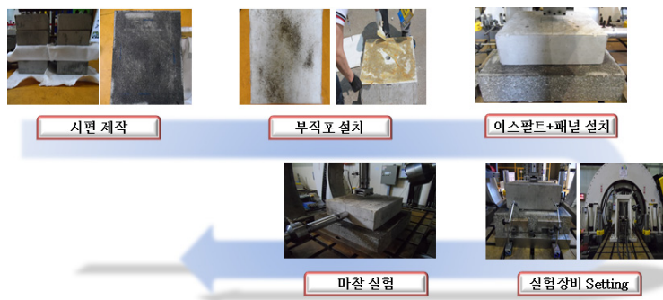
Figure 1 Process of Friction Test
