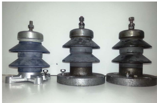
Fig. 3 Photographs of lightning arresters
