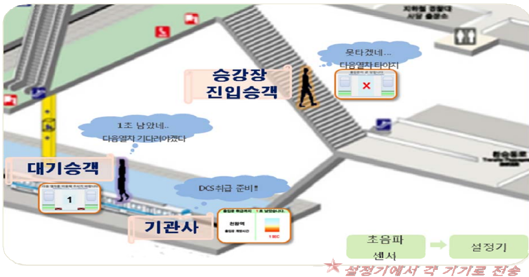
Fig. 2 Doors closing time notice system operating configuration
