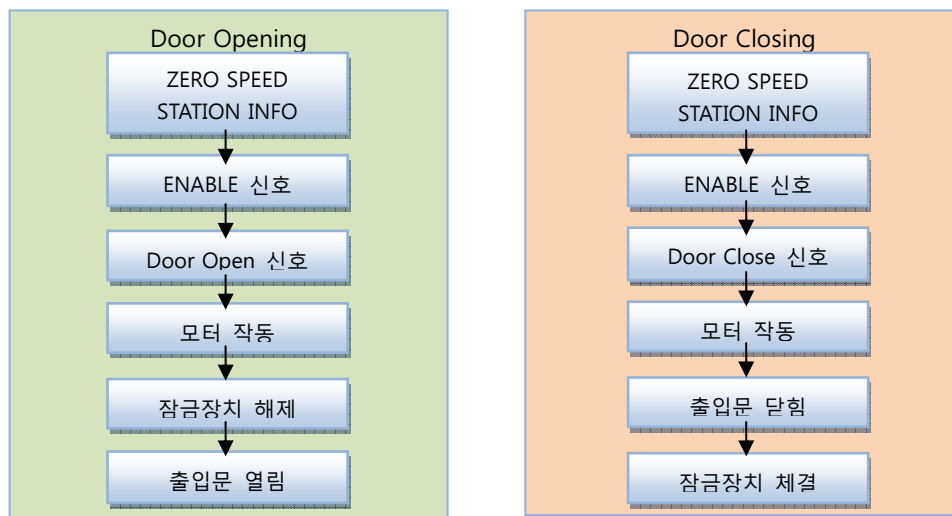
Fig. 1. Flowchart of EMU door operation
