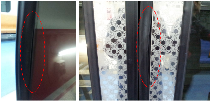
Fig. 9. Falling of Edge Rubber
