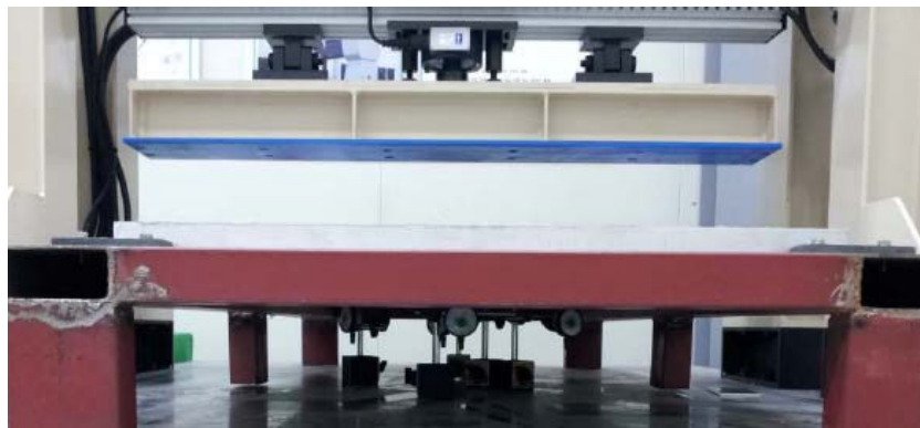
Fig. 4 Alternating load test Machine and Measuring Gauge
