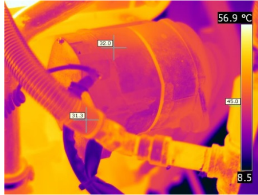
(b) Auxiliary power generator in shunting locomotive
