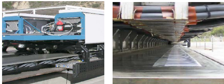
Fig. 4 Position detection system for GA[4]
