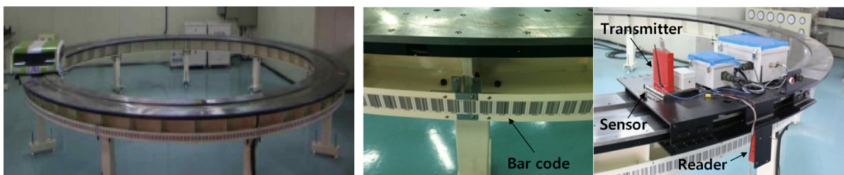
Fig. 5 Barcode position detection system[5]
